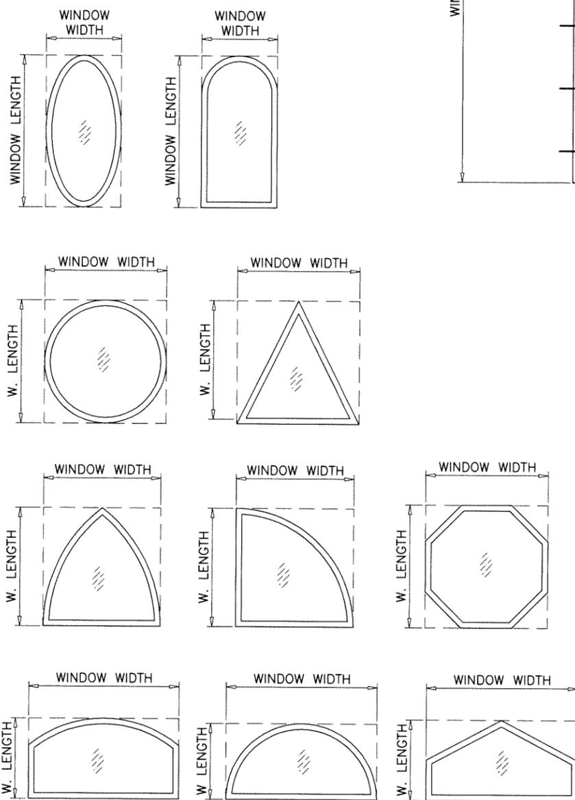
ALLOWABLE LOADS FOR ALTERNATE SHAPES AS SHOWN ABOVE OR SIMILAR CAN BE VERIFIED BY INSCRIBING PICTURE WINDOW SHAPE WITHIN SQUARE OR RECTANGLE AS SHOWN IN DOTTED LINES AND OBTAINING ALLOWABLE LOADS FROM THOSE SHAPES.
